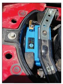
Featherweight batteries by Western Power Sports not only produce more cold-cranking amperage and have a much longer lifespan than lead-acid batteries, the lithium-ion batteries weigh half as much and have a charge indicator embedded in the plastic case. Remove your seat and press the "test" button to check the charge level.
